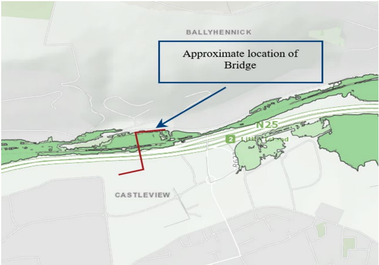
Image 2.3: Extract from South Western CFRAMS coastal flood extents, current scenario (0.5% AEP)
